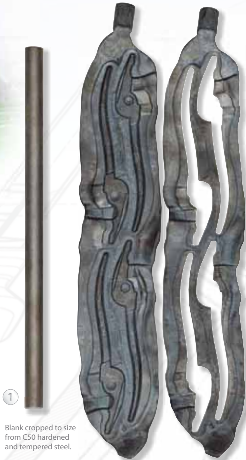
2 Hot forged in the double forging die. The excess burr is removed under an eccentric press.
