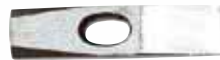
6 After descaling the blank, it is machined all round in accordance with DIN 1193. The pein and face of the hammer head are additionally ground.
