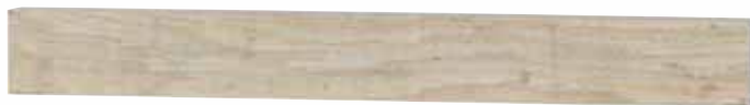
1 Shaft blank from hickory. This tough wood has long fibres, making it ideal for hammer shafts. The long fibres cushion the impact in the hand. The tight annealed rings give the wood its flexural strength.
