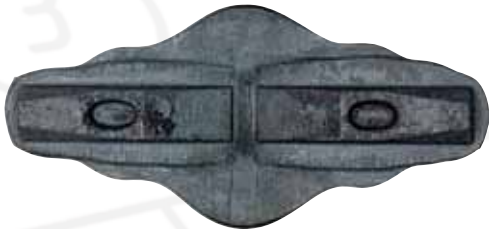
3 Fully forged blank.
