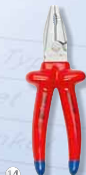
14 The plastic coating on the handles is built up by multiple dipping in liquid immersion compound.
