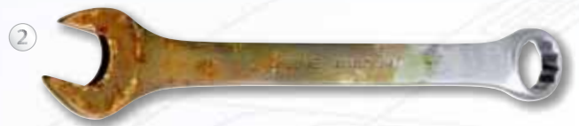
2 The surface has clear traces of rust film
