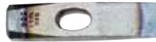
7 The hammer head is induction hardened to 50-58 HRC and then annealed. Care has to be taken to ensure that, within a defined measured area, the hardness deviation is no greater than 5 HRC. The hardening depth on the face and pein must be at least 3 mm. The hardness of the eye zones, however, must not exceed 30 HRC. The hammer head now has hard striking faces and a soft "shock absorber" zone. These safety-relevant values are subject to continuous monitoring. The hammer head is permanently stamped with the manufacturer's mark, weight and DIN 1041.
