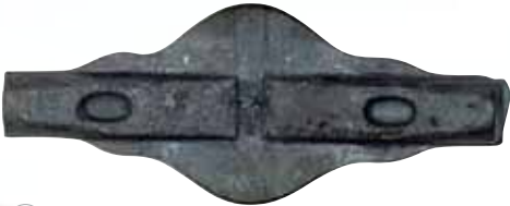
2 Hot pre-forged in a double forging die.
