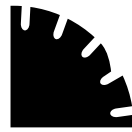
C1S Wide spacing, wide slots. Protected with a drop wear segment to guard against the undercutting effect
