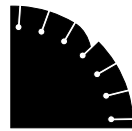
C3S Close spacing, narrow slots with hole slot. Protected with a drop wear segment to guard against the undercutting effect
